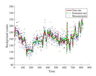
Figure 9: Using the Kalman filter to estimate the background rates from noisy measurements in an energy bin.
