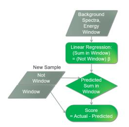
Figure 3: The CEW detection algorithm.
