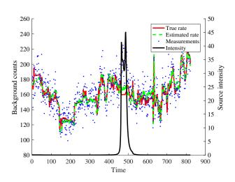
Figure 15: Using the adaptive Kalman filter to estimate the background rates in an energy bin in the presence of a source.
