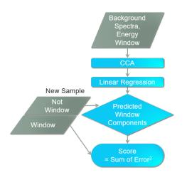
Figure 5: The CCA detection algorithm.
