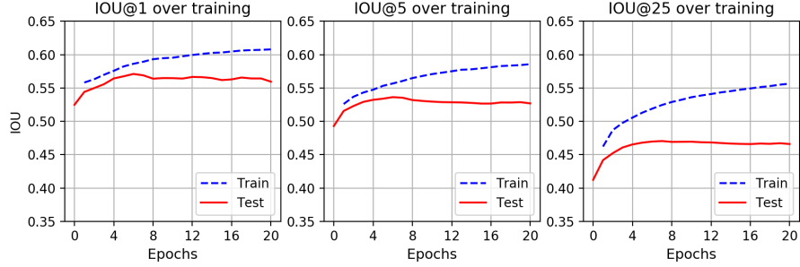
Figure 4: Training and testing curves over epochs trained during finetuning. From left to right, plots show the IOU of the system averaged over 1, 5, and 25 frames ahead of the key frame.
