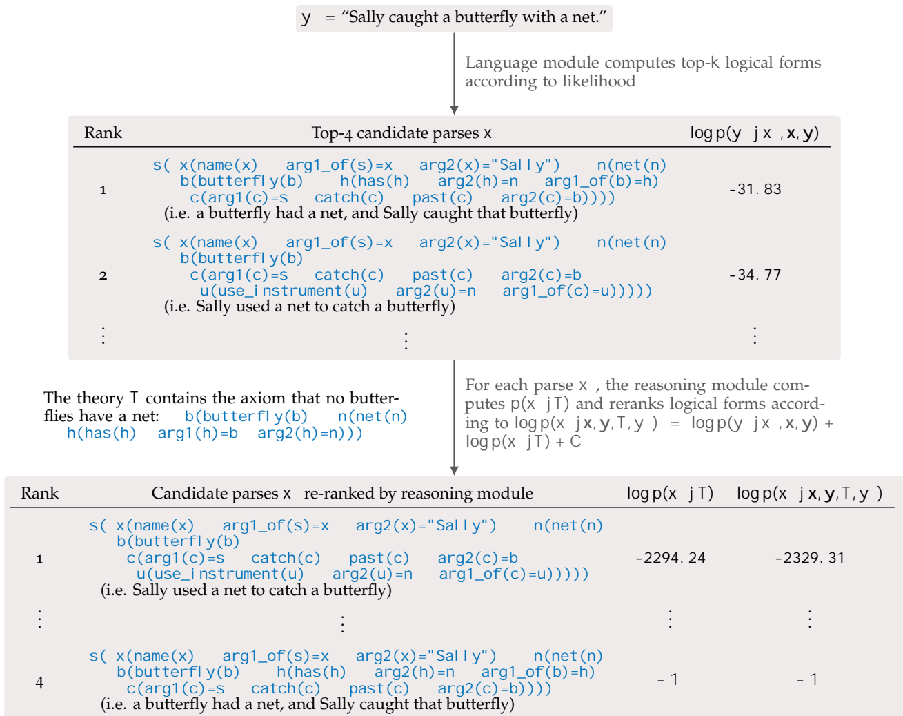
Figure 21: An example where PWL reads the sentence “Sally caught a butterfly with a net,” which is a classical example of a sentence with prepositional phrase attachment ambiguity: “with a net” could either attach to “butterfly” or “caught.” In PWL, “reading” a sentence is divided into two stages: (1) find the 4 most likely logical forms, ignoring the prior probability of each logical form conditioned on the theory, and (2) for each logical form in the list, computing its prior probability conditioned on the theory and then re-ranking the list accordingly. The output of the first stage is shown in the top table, and the output of the second stage is shown in the bottom table. In this example, PWL has previously read “No butterfly has a net,” and added its logical form to the theory. As a result, the reasoning module is unable to find a theory that explains the logical form where the butterfly has the net, and so the prior probability of that logical form is zero. The log probabilities in the bottom table are unnormalized.
